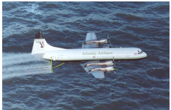
Figure 2: Dispersant spraying (source: Mark Kirby)
